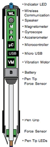
Figure 1: Potential design of Pika Pen showing feature set.
