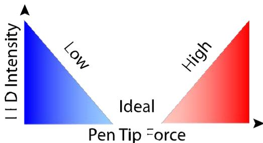
Figure 3: Pen tip force indicating mode where two LED's communicate the ideal force. Different colors and intensity indicate direction and amount of force applied.
